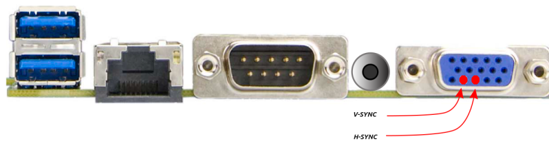
Figure 4.1: Mechanical Disablement Points on VGA Connector (Pins 13-14)
